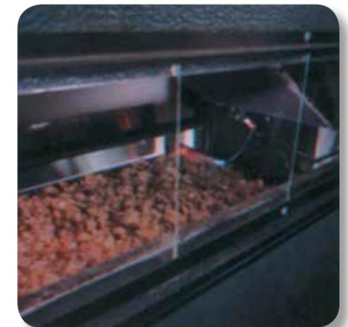
Fiber glass loosefill and batt insulations pass the ASTM E970 fire safety test.
